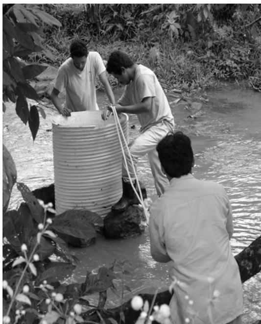
**Figure 2.** Open cylinder used to measure flow across the river sediment. Blocks are placed on top of sandbags resting on a tire inner tube placed around the cylinder to seal it to the bottom. The installation is adjusted to minimize the Venturi/Bernoulli effect anticipated under the turbulent river flow conditions.
