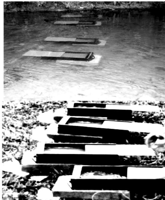
**Figure 2.** Sediment traps used for the gross accumulation and sediment resuspension assay in the Sucio river.
