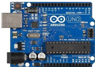
Figura 7: Arduino Uno R3 DIP
