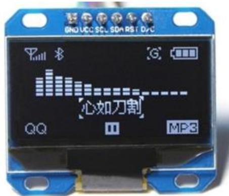
Fig.3.2(a): Display OLED 128x64
