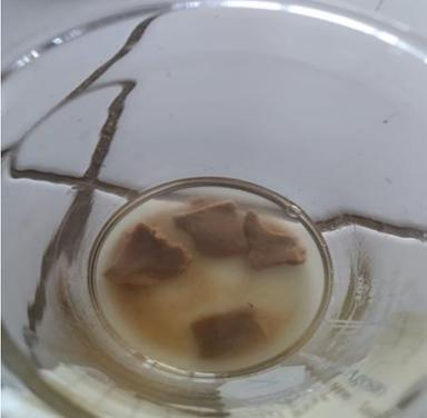
A petri dish containing a larger amount of dark brown, solid material, showing further biodegradation after 10 days.                 |
