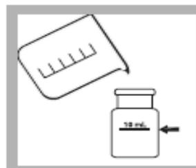
3. **Prepared Sample:** Fill a clean square sample cell with 10 mL of sample.
