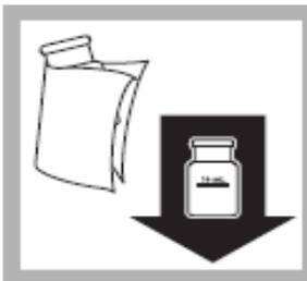
10. Within eight minutes after the timer expires, insert the sample into the cell holder with the fill line facing the user.
