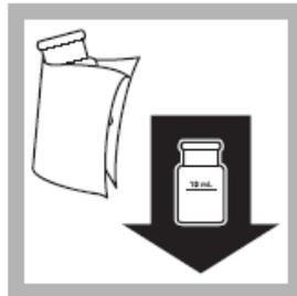
**10.** Wipe the blank and insert it into the cell holder with the fill line facing the user.
