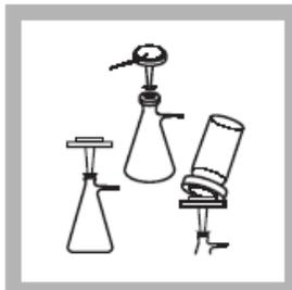
4. Assemble the filtering apparatus (0.45 micron membrane filter, filter holder, filter flask, and aspirator).
