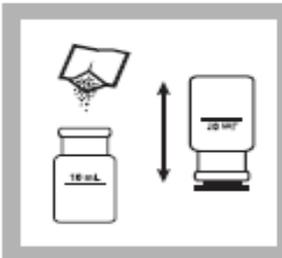
5. Add the contents of one Sodium Periodate Powder Pillow to the sample cell. Stopper and invert to mix.
